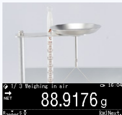
First measure the empty weight.
