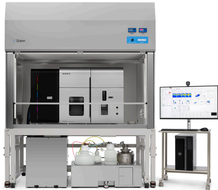
Figure 9 – FP7000 Spectral Cell Sorter inside custom class A2 level II Biosafety Cabinet
